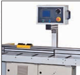
Outfeed roller table (auto- matic positioning system)
