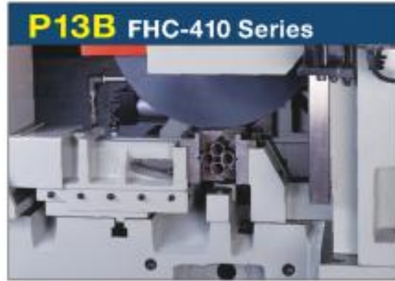
P13B FHC-410 Series V型夾鉗多支式。 Multiple "V" vise.
