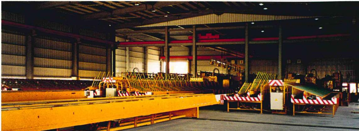
High capacity shear-line that allows to reach a **very high production**, reducing dead times to a minimum, immediately clearing the cut material and start directly the following working cycle. Particularly suitable for **large standard productions**, it can also be adapted to reduced spaces.
