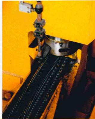
It is the smallest shear of the cutting range but, however, allows to cut bars with a diameter up to 55 mm.
