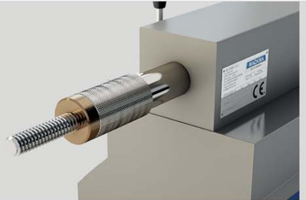
Simple mechanical locking screw for bend stop position
