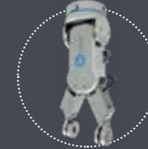
RG2-FT Smart gripper with proximity and force/torque sensors
